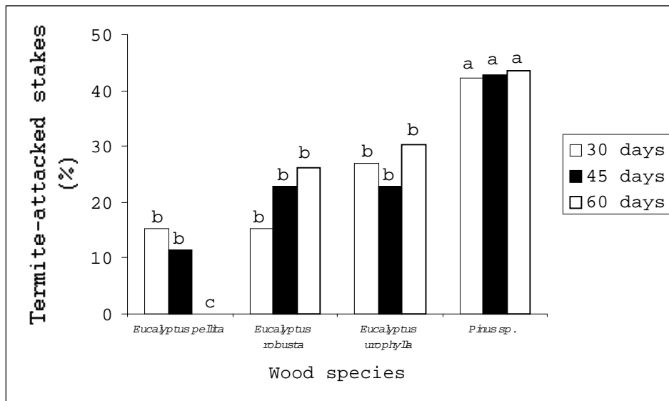
Figure 1. Percentage of stakes of each wood species attacked by subterranean termites at 30, 45, and 60 day exposure periods in the field in Seropedica, RJ. Averages within the same exposure period followed by the same letter are not significantly different as gauged by Tukey’s test ( P \leq 0.05 ).
