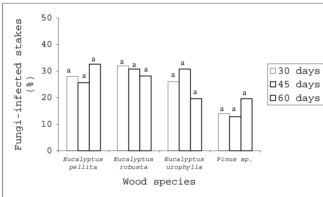
Figure 2. Percentage of stakes of each wood species infested by basidiomycetes fungi at 30, 45, and 60 day exposure periods in the field in Seropedica, RJ. Averages within the same exposure period followed by the same letter are not significantly different as gauged by Tukey’s test ( P \leq 0.05 ).
